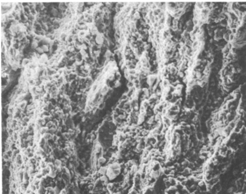
Figure 9 SEM fractograph of intergranular fracture in necklace Rene 95, \times 500 .
