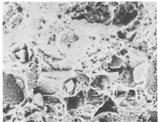
Figure 12 Fracture surface in a vacuum stress rupture test. Necklace Rene 95, \times 500 .
